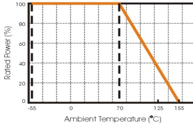
Fig.2 Maximum dissipation in percentage of rated power
