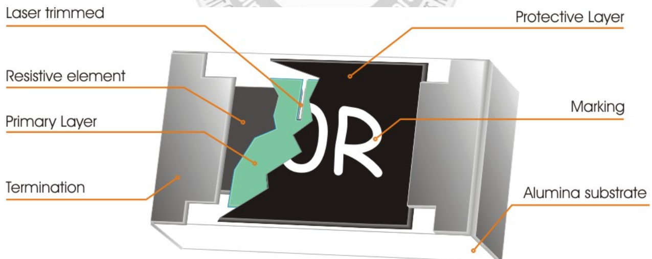
Fig 1. Construction of Chip-R WFxxK
